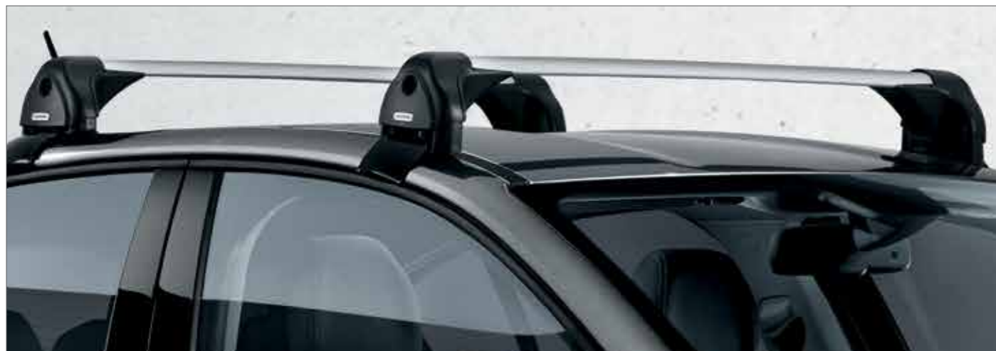
ROOF BARS - TIPO 5DOOR - 52046032 To be installed directly on the roof. Max Load Capacity: 50 Kg.
